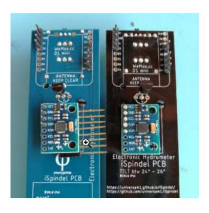
1) Use a female pin header as spacer, it's necessary when the gy 521 module must be welded. This way to ensure correct alignment with the horizontal plane.
