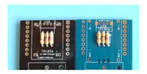
1) Assembling resistances places on battery holder side  $1 = 230K\Omega$ ;  $2 = 330\Omega$  or BAT43 diode; 3 = 4K7
