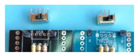
1) Solder to slide switch Attention = only for 2.1 PCB version, please cut the pins of the external frame of the sliding switch
