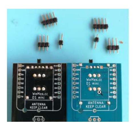
1) For mounting wemos module it's not necessary to weld all the pins, but only those interested. Prepare the pieces 1x4 pin, 1x1 pin, 1x3 pin as picture
