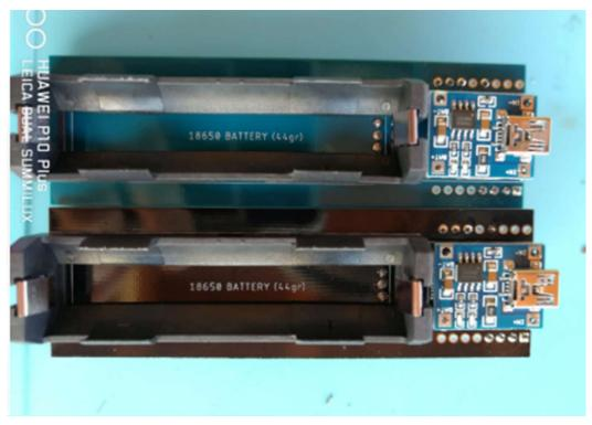
Rotate pcb on bottom side and places the battery holder before and tp4056 module after
